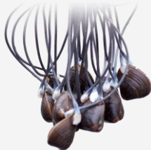
Live biomonitoring using bivalves for real-time water quality assessment
